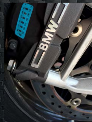
Brake caliper prepared with temperature stickers.
