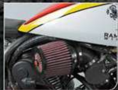
XSTREAM® SERIES AIR FILTER INSTALLED
