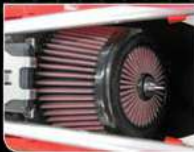
XSTREAM® SERIES AIR FILTER INSTALLED
