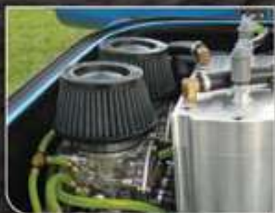
FLAME ARRESTOR #59-2046 INSTALLED
