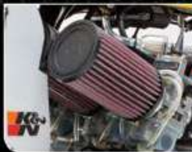
SPECIALTY CLAMP-ON AIR FILTERS INSTALLED
