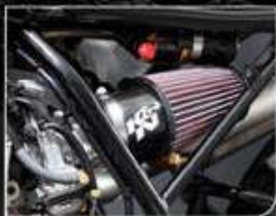
PLIABLE MOLDED FLANGES ABSORB VIBRATION
