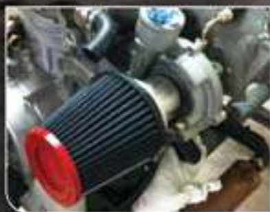
FLAME ARRESTOR #59-2040RR INSTALLED
