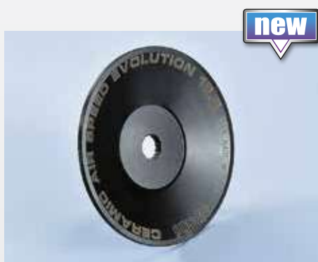
244.0128 Yamaha fixed ceramized halfpulley 12,5° Semipuleggia fissa ceramicata 12,5°
