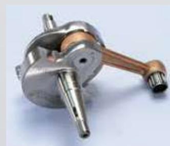
210.0043 Vespa PX125 advanced/anticipato, stroke/corsa 57
