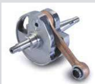
210.0042 Vespa PE200 advanced/anticipato, stroke/corsa 60
