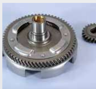
202.1219 Vespa 75/100 Z=22/63 Primary ratio-Primario
