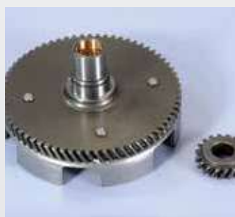
202.1218 Vespa 50/75 Z=18/67 Primary ratio-Primario
